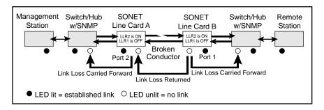
**IMPORTANT:** LLR must not be active on both ends of a configuration. If it is, the link can never be established.
